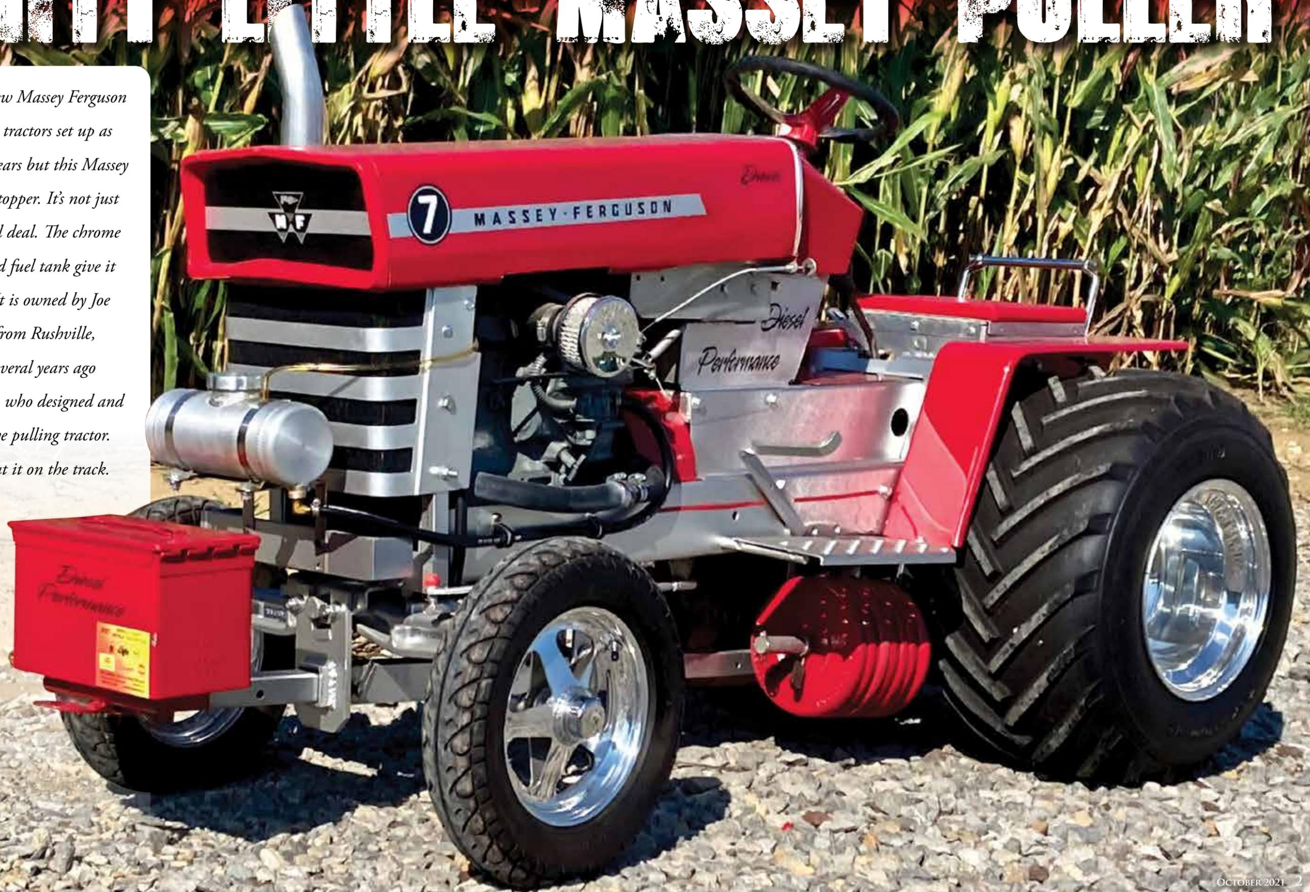
It is powered by a Kubota three-cylinder diesel engine which is mounted backwards in the tractor frame. That means the transmission is run by the drive shaft that originally powered the mower deck in a standard Kubota lawn tractor. I have used a Kubota lawn tractor with that same three-cylinder diesel engine for over thirty years and they are a real powerhouse. The engine has 1,600 hours and doesn't burn a drop of oil.
