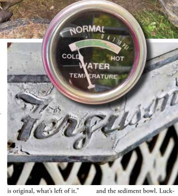
A few years ago, Roger was doing some repair work on the Ferguson and had purchased a new radiator that did not fit quite the same as the old one. That meant the original grille would not fit over the radiator, so he fashioned a new grille out of expanded metal which he cut, bent and shaped to fit. The replacement grille seemed to work pretty well. At the same time, he replaced the fuel tank
